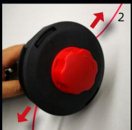
Pull the line on both ends
