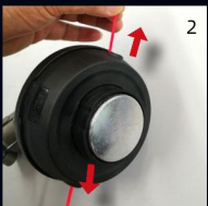
Pull the line on both ends
